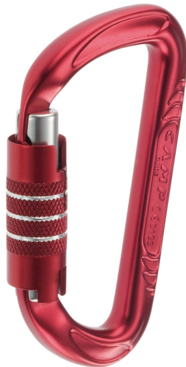
Automatic lock requires three actions: slide, twist and open.
